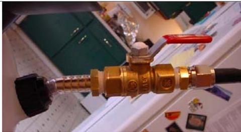
Thing™'s valve to fill it with beer. When it's filled, shut the valve and screw a picnic tap beer hose to the flare
