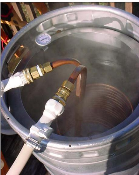
coils, it picks up heat from the surrounding water, and goes back to the top of the mash a little warmer than when it came out the bottom of the mash.
