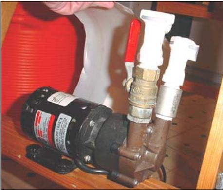
Close-up of the March pump with the splash shield pulled back. The valve which controls the pump's flow has to be installed on the OUT port of the pump.
