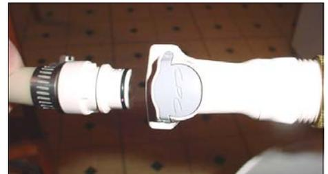
Brewer), but I went to the source and found a wider variety of fitting options at better prices. Look for the "HFC" line of plastic connectors at [www.quickcouplings.net](http://www.quickcouplings.net). They snap together with a positive "click", and easily separate again with a press of the button on the "female" coupling.
