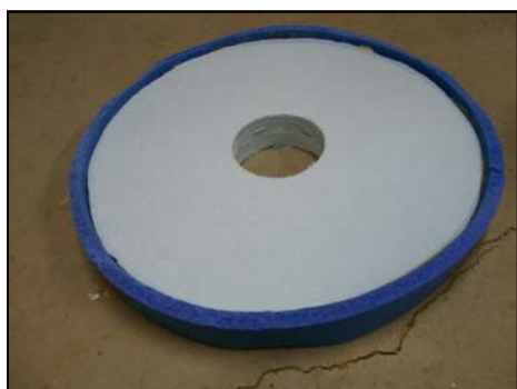
The 13" diameter jacket lid was cut from Styrofoam board insulation with a strip of sleeping pad foam glued around its perimeter. The center hole allows the air lock to protrude.
