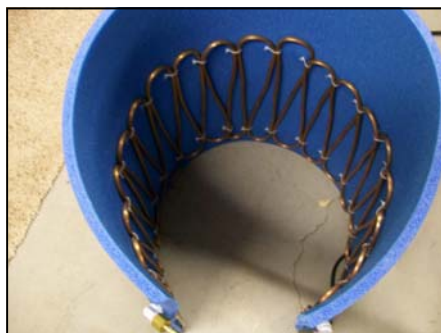
The full length of copper tubing is shown here attached to the foam pad. The foam will help retain the cold when the copper coil is placed around the fermentor.
