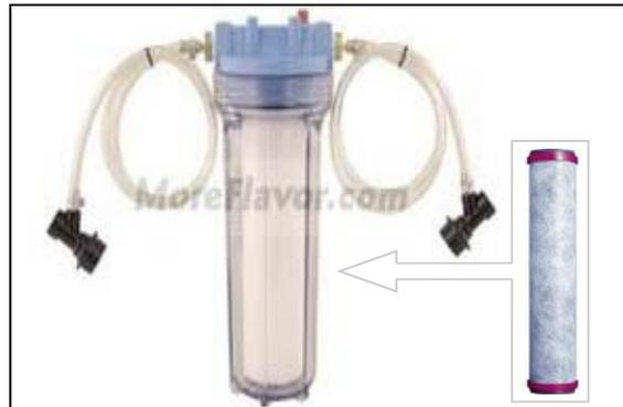
For water supplies which use chloramine, a carbon filter will remove it, but it requires longer contact time with the carbon. In this case, the rate of flow through the filter should be less than one gallon per minute, which is like a trickle. If you have the time, fine. If you don't have the time, and your water is treated with
