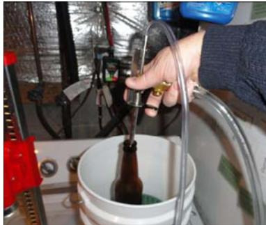
The BeerGun is extremely simple to break down without tools for cleaning after use. The manufacturer recommends only hand-tightening the nut which holds the stainless steel nozzles to the handle. They also recommend taking the handle apart. But because no beer flows through the handle, I have not yet seen the need to clean it out or take it apart.
